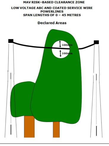
The minimum clearance space for foliage around Uninsulated Low Voltage and High Voltage ABC cables using the risk-based management approach is 300mm. Foliage within 300mm of Uninsulated LV and HV ABC or likely to grow within 300mm within the next inspection period will have a high risk score.
